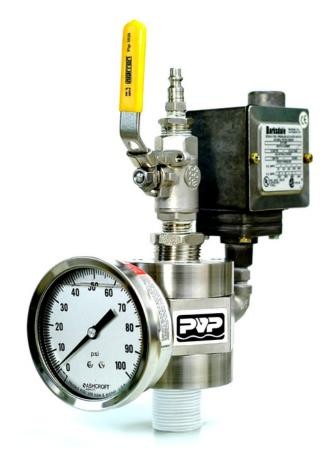
The model 420 vacuum and pressure sensing assembly was designed to provide protection for the Double Disc Pump<sup>™</sup> line of positive displacement pumps manufactured by Penn Valley Pump Co.,Inc. Our vast experience in pumping and hydraulics has led to a protective device that surpasses those previously available. This device provides protection against the inadvertent pumping against a closed valve or a blocked line thereby preventing damage to the pump.
