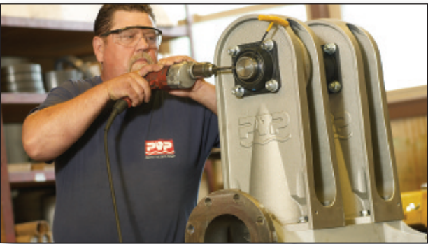
Figure 20. Assembly of a Model 6DDSX76 pedestal bearing and drive shaft.
