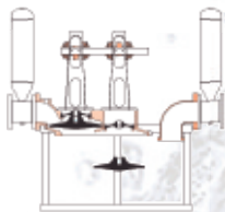
Figure 12. Suction disc removed after removal of suction housing. Easy access given clearance under frame.
